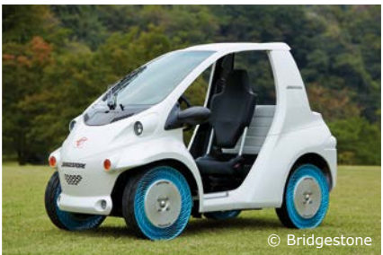
Reinventing the wheel The innovative idea of airless tires can be extended to cars as well
