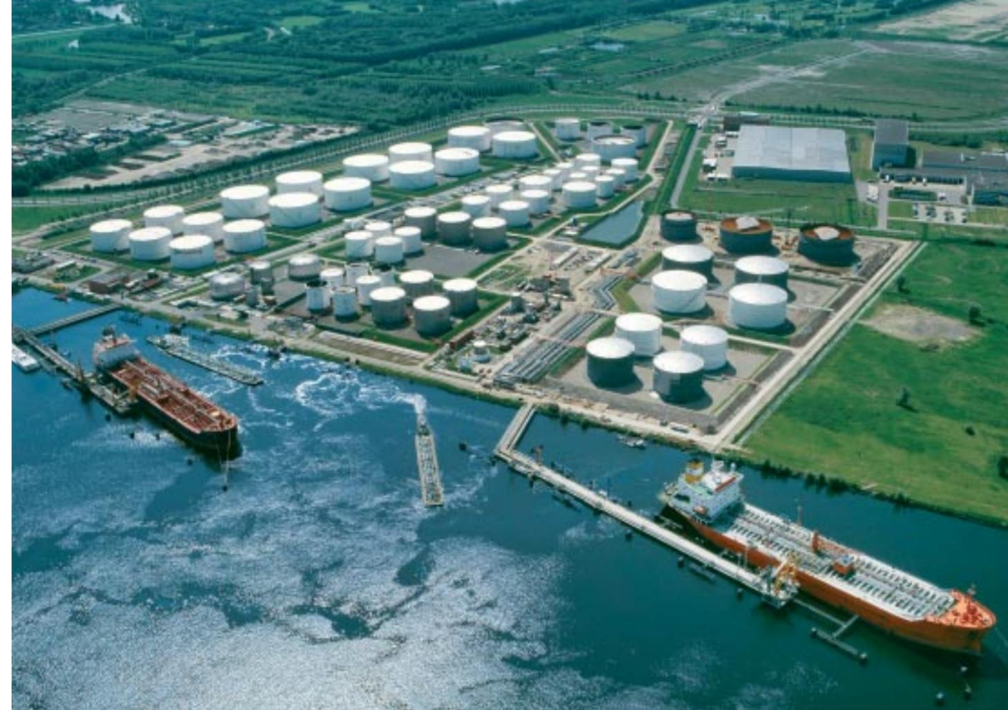
The Oiltanking Amsterdam terminal: With the new tanks the tank capacity grew with 34 percent. The new jetties increased its capacity by 40 percent.
